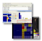
The Calibre nmDRC-Recon DRC Analyze function enables fast, in-depth visualization and analysis during error review and debugging.
