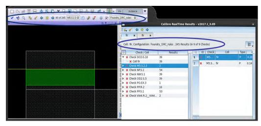
Designers can highlight results using either the Calibre RealTime Custom toolbar or the Calibre RealTime Custom results window.
