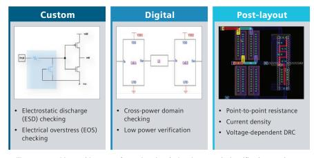
Calibre PERC enables a wide range of complex electrical and geometrical verification requirements to ensure product reliability and performance.
