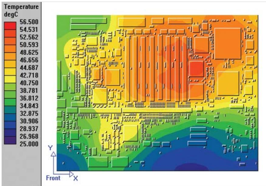
HyperLynx Thermal allows engineers and PCB designers to analyze board-level thermal problems on placed, partially routed, or fully routed PCB designs from all popular PCB layout environments. Temperature profiles, gradients, and excess temperature maps enable designers to resolve board and component overheating early in the design process.
