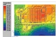
high-power requirements, for example, but the surrounding board is reasonably cool, a thicker reference plane may provide the solution. If the board surrounding the hot component also has a high temperature, other heat transfer solutions can be employed.
