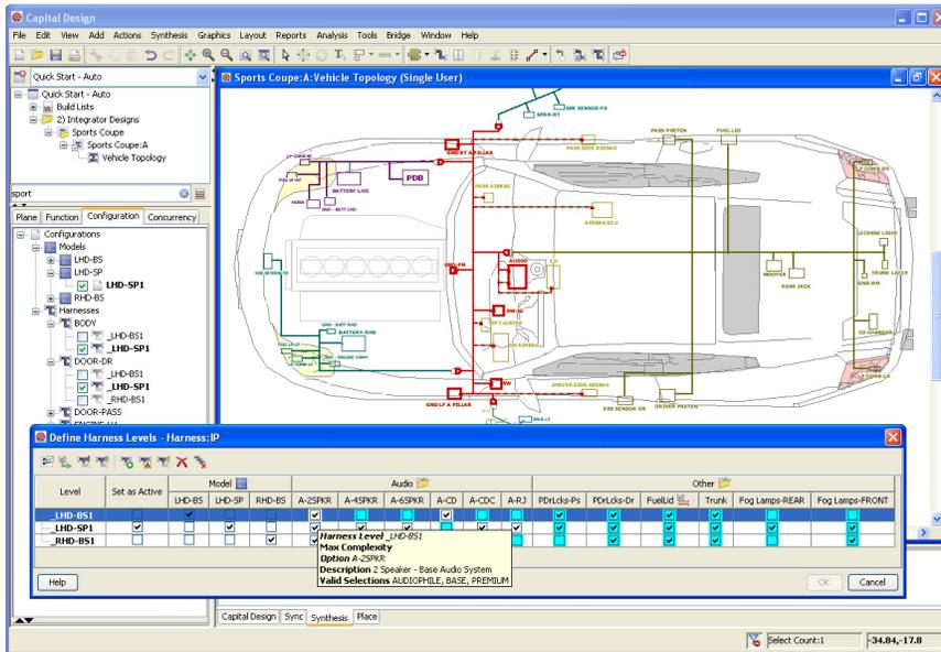
*Generate wiring designs and diagrams automatically from physical layout, system designs, and option content*
