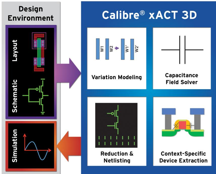
Calibre xACT 3D provides a complete parasitic extraction solution with deterministic field solver accuracy, process variation modeling, electrically aware reduction, and industry-standard netlist formats, all within the design environment.
