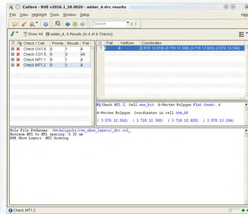
The Calibre RVE interface allows users to automatically display DRC check-relevant layers in the design environment using the CTO file.
