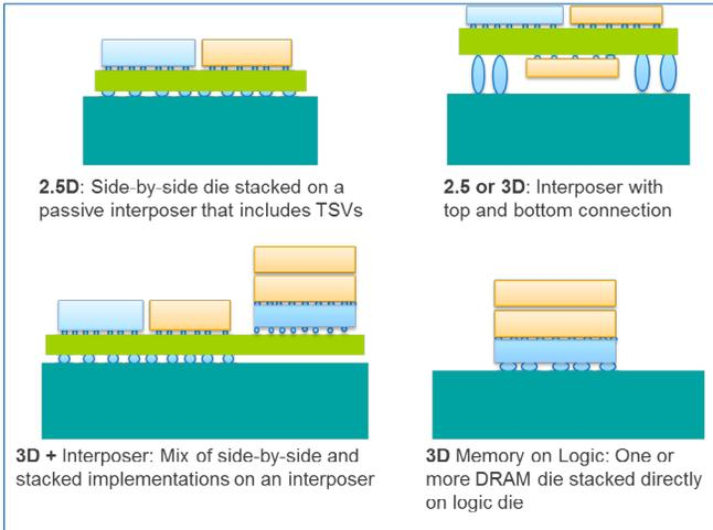
Typical 2.5D and 3D configurations that Calibre 3DSTACK can support.
