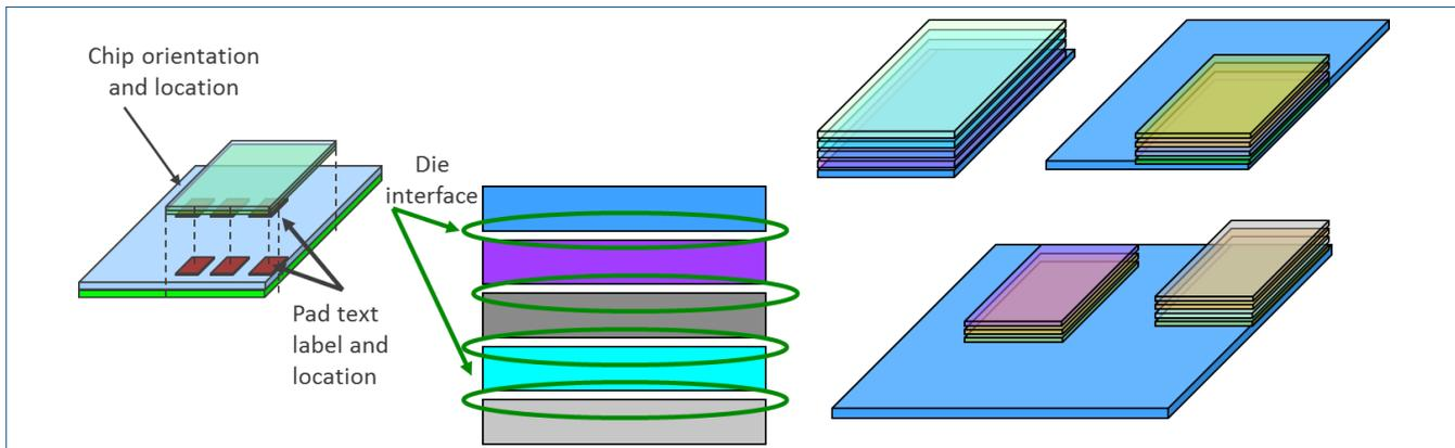
Calibre 3DSTACK uses information supplied in the rule deck to support the various stacking configurations.
