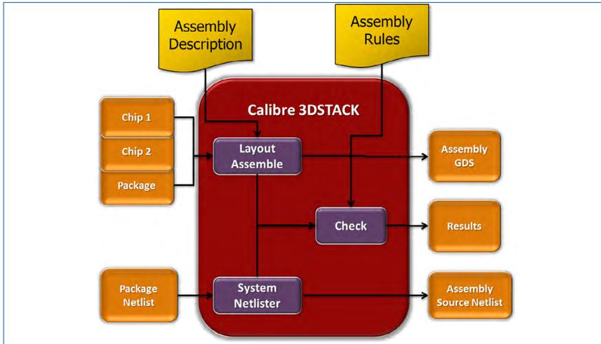
Calibre 3DSTACK enables signoff verification of chip stacks with flip chips, silicon interposers, through-silicon vias, and more.
